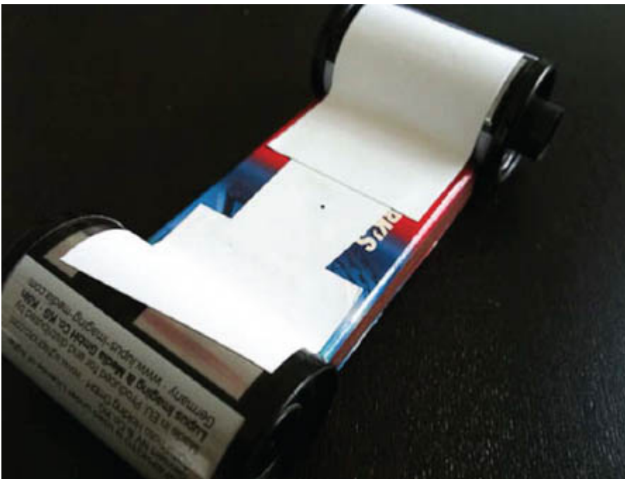
Figure A-9: Use tape to lightproof the camera. The only place where light should enter is through the pinhole.
