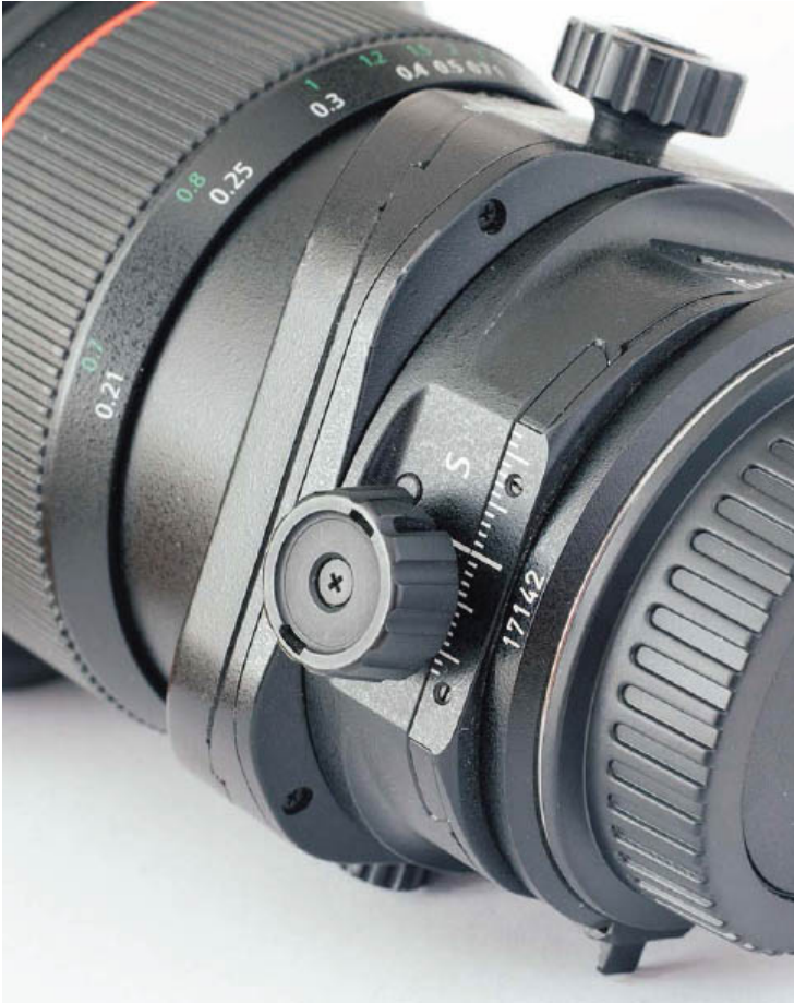
Figure 6-12: Shift functionality is controlled using a knurled knob. The locking screw is on the opposite side of the lens body.
