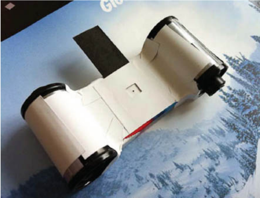
Figure A-10: A slider made of black cardstock serves as a shutter.
