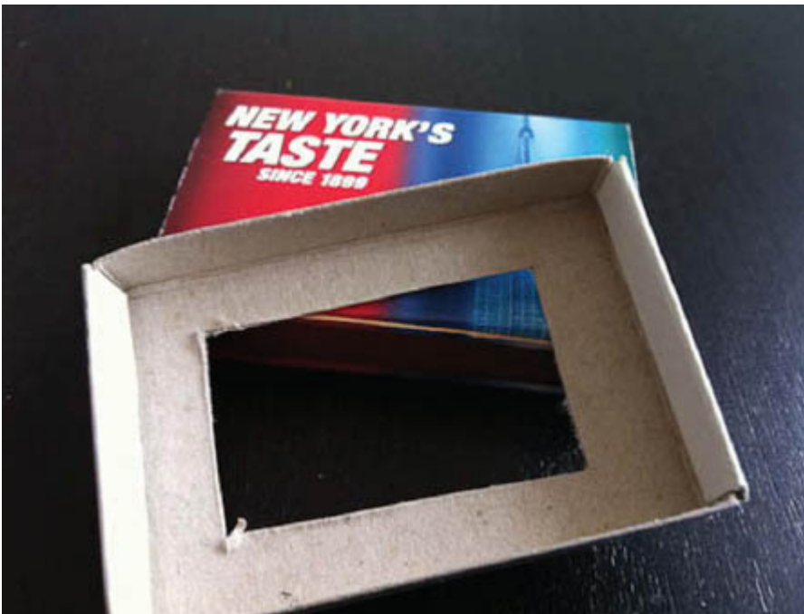
Figure A-3: The drawer of the matchbox is transformed into a film carrier.
