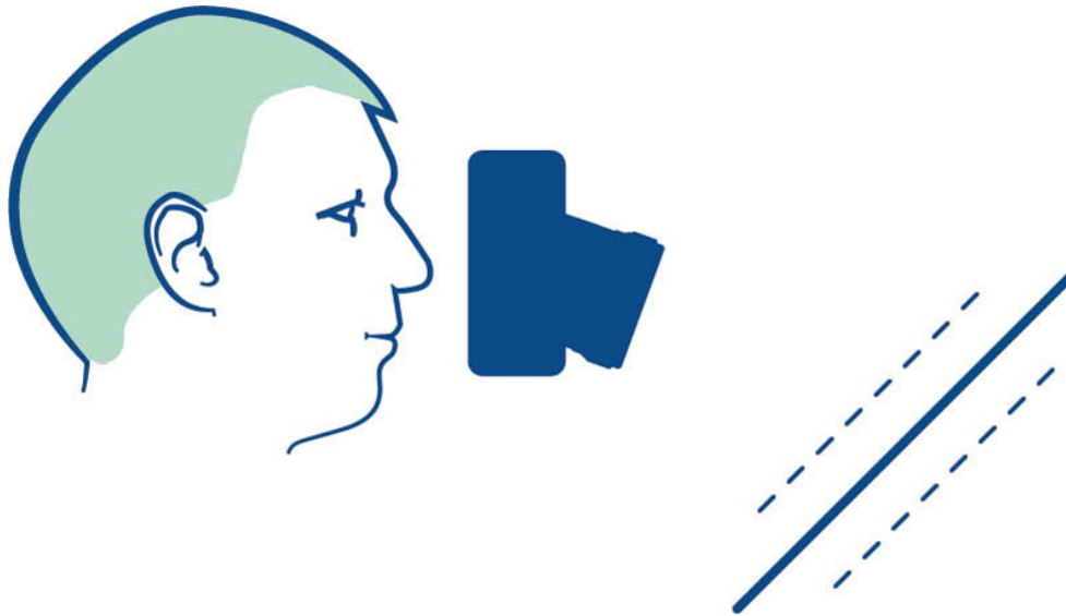
Figure 7-13: Tilting the lens tilts the plane of focus. Tilting the lens forward makes the depth of field gradient run from bottom to top in the image, rather than from near to far, as is usually the case.
