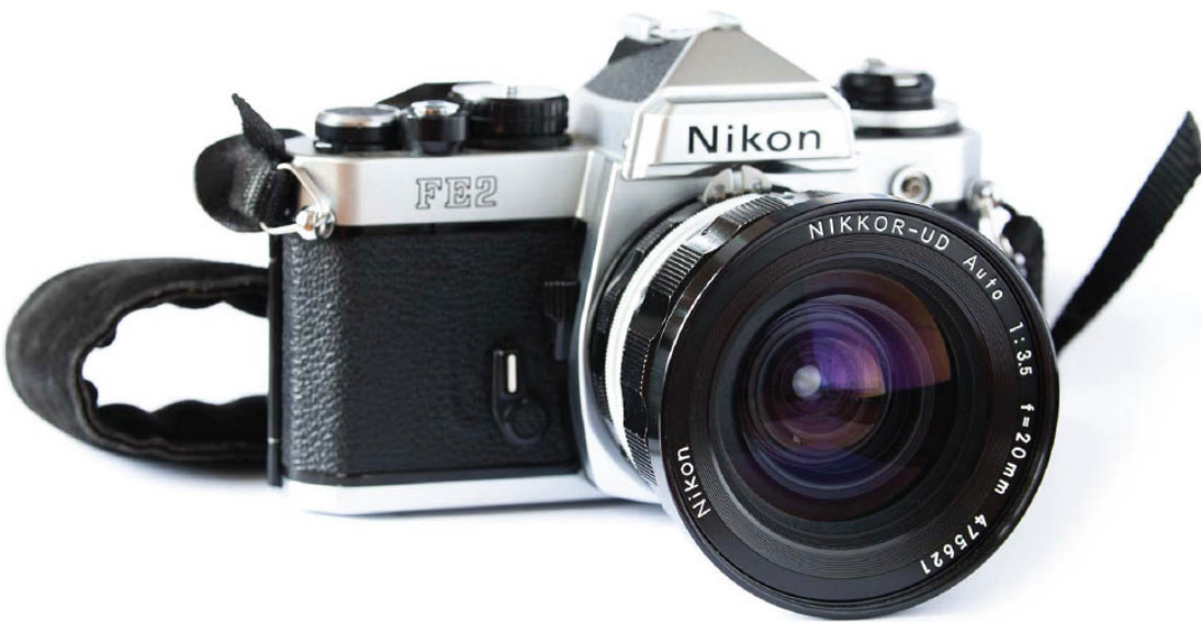
Figure 1-2: An analog Nikon FE2 fitted with a 20mm wide-angle lens.
