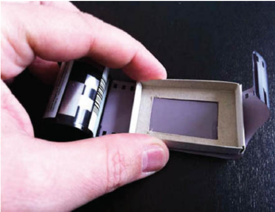
Figure A-5: The width of the matchbox fits the width of the film, which is exposed through the rectangle cut into the bottom of the drawer.
